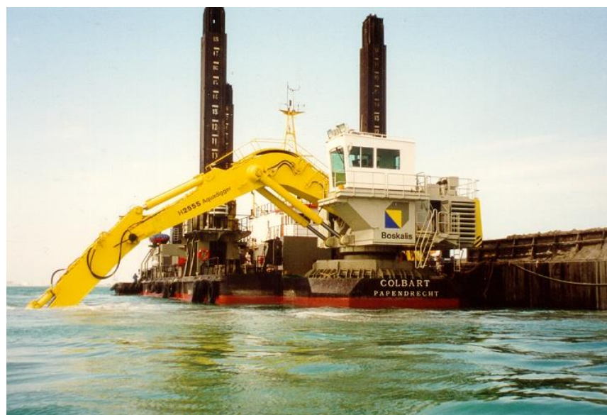
Figure A17. 2 Backhoe Dredger (Source: Boskalis)
