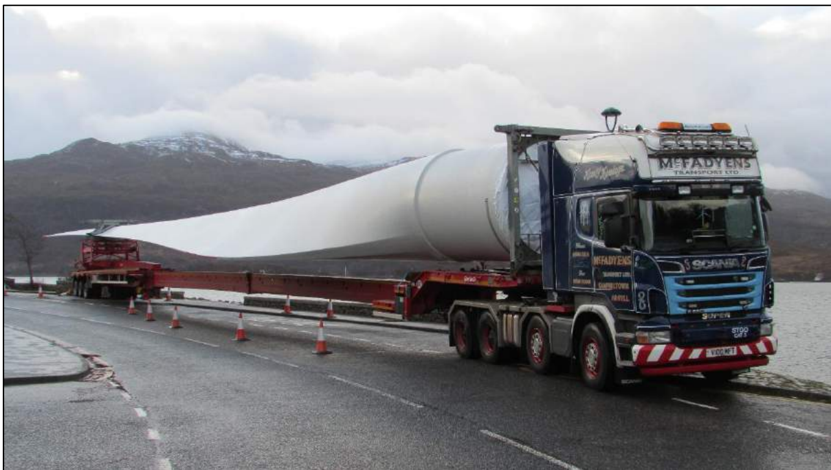
Photograph 1 - Super Wing Carrier carrying Turbine Blade
