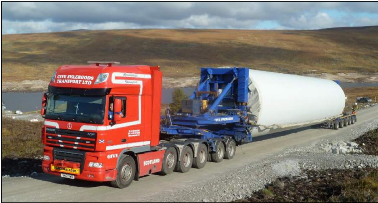
Photograph 2 - Base Tower Transport
