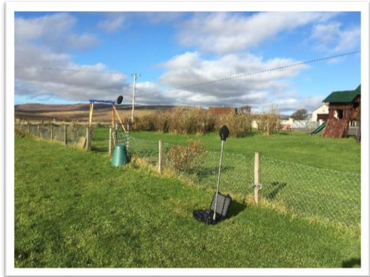
Figure 5: Noise surveying equipment
